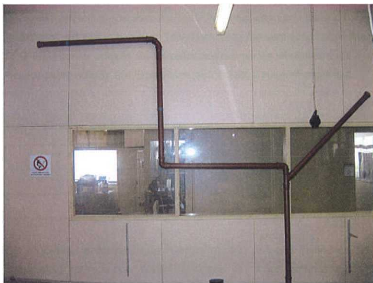
Fig. 1: Test set-up for tightness against negative pressure
