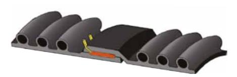
Integrated wire in the socketed end. Joining by electric fusion welding. Shorter sockets, increased overall effective pipe length, secure and watertight connection.
