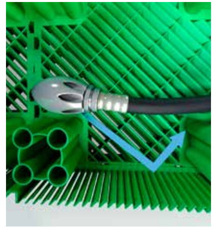
Innovative construction of side panels and bottom plates - inclined ribbing, which during cleaning reverts the pressure water jet and prevents damage to the geotextile.
