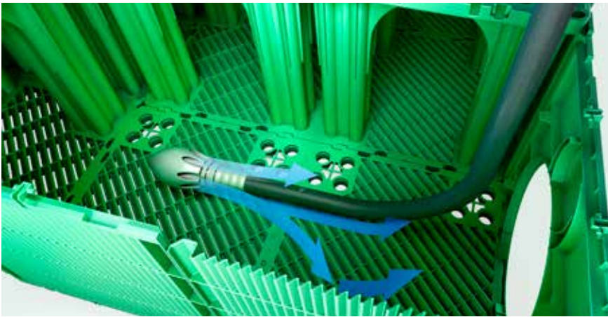
Innovative construction of side panels and bottom plates - inclined ribbing, which during cleaning reverts the pressure water jet and prevents damage to the geotextile.
