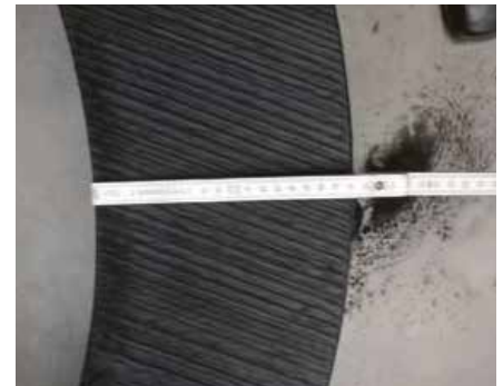
Solid wall pipe made of polyethylene s = 180 mm
